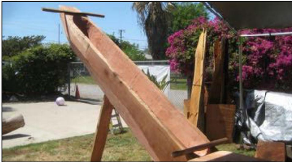
Setting the bow was the trickiest due to the tight alignment tolerances from one bow to the other. With a simple string and a plumb bob we found the center ... exactly the same procedure used centuries ago by boat builders of old.
